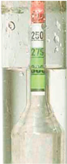
Figure 1.59 Measuring relative density with a hydrometer
